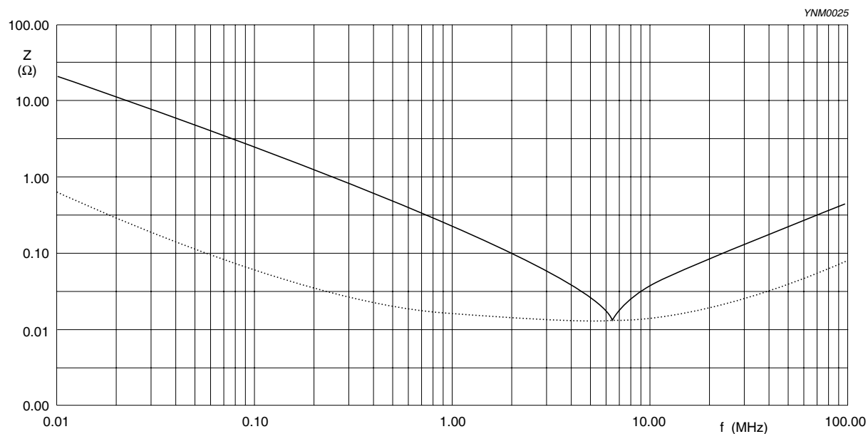
Fig. 7 Impedance ESR vs. frequency characteristics for multilayer chip capacitors
